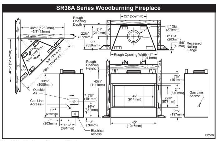
Fig. 1 SR36A Series specifications and framing.
